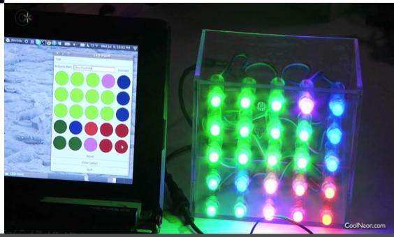
Individually programmable LED lights will make up the "pixels" on the LED screen. A controller will cycle through the phases of the moon. An Arduino lighting program with multiple years worth of moon phase and sun revolutions can be supplied as part of the original artwork.
